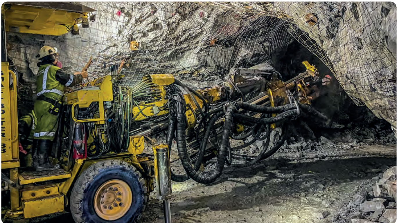
Electro hydraulic drilling rig
